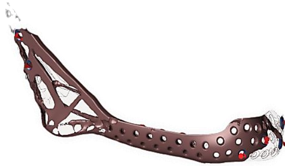
Figure 4. Topologically optimized part
