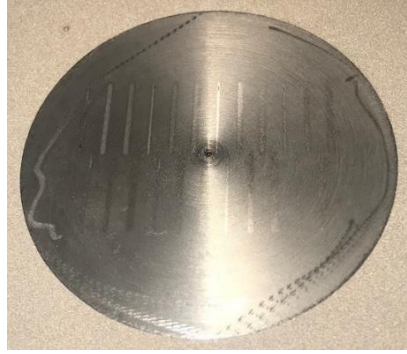
Figure 1. Picture Showing Powderless Single Track Experiment Without Preheating
