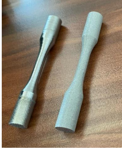
Figure 2. The appearance of fatigue samples before and after the electrochemical polishing process.
